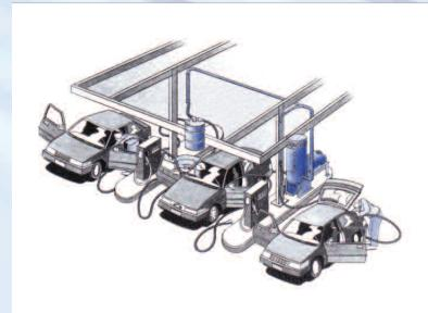
The vacuum unit can be installed on a gasoline island by using an explosion-proof motor and controls, grounded hose, grounded filter bags and a metal tubing system, all available from Spencer.
