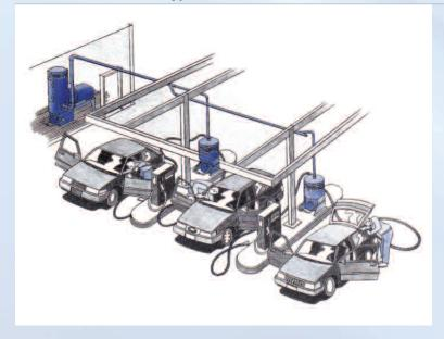
This approach saves space by moving the unit away from the gasoline island. Grounded hose, grounded filter bags and a metal tubing system are required. All are available from Spencer.
