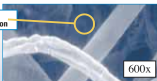
Conventional media has spaces of up to 60 microns between the fibres, allowing dust to become deeply embedded.
