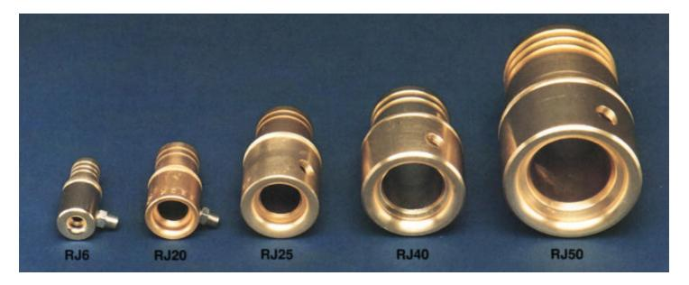
Pneuvay Engineering's Ringjets utilize in-shop compressed air and employ a venture-type design which induces air to flow in through the throat.
